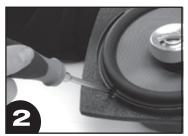
To install speaker wire it may be necessary to penetrate the baffle housing to route the wire.
